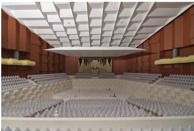
Figure 8: Picture of the 1:10 scale model of De Doelen with the new suspended technical ceiling above stage. In this ceiling the reflectors and lighting is integrated.
