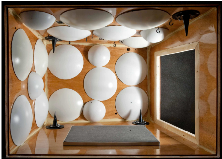
Figures 10 and 11. Scale model reverberation room with panel diffusers and carpet specimen (top) and volume diffusers with foam specimen (bottom).
