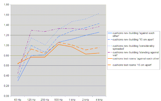
Figure 9: Sound absorption per \text{m}^2 element of broadband absorber applied in the Conservatorium van Amsterdam
